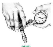
Pilot tube shown properly inserted into sprinkler nozzle.
